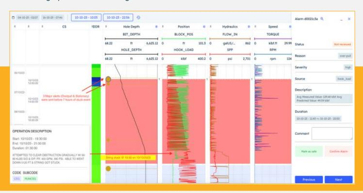
Information that is aggregated by DRILLTECT is sourced from surface sensor data, including depth, flow, pressure, and rotation. The ability to detect subsurface anomalies early is a key feature and benefit of DRILLTECT.
