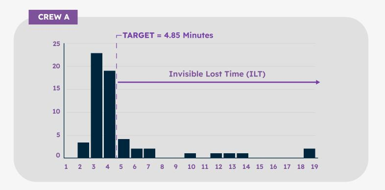
ILT is a good measure of drilling efficiency, though it requires a reference performance against which to measure the gap from current performance.
